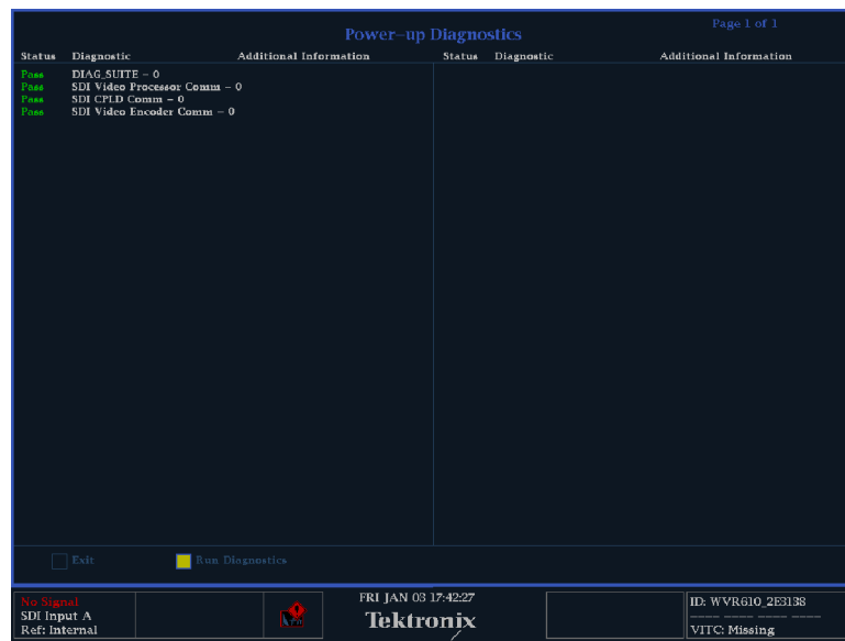
Figure 2-52: Power-up diagnostics passed
