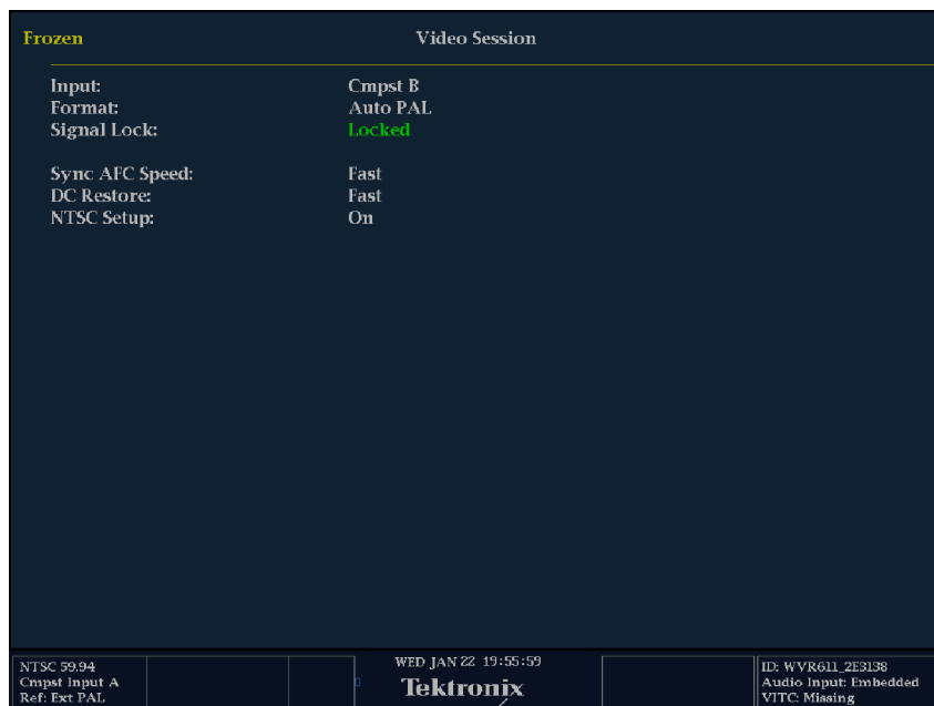
Figure 3-25: Video session status display for a CMPST input
