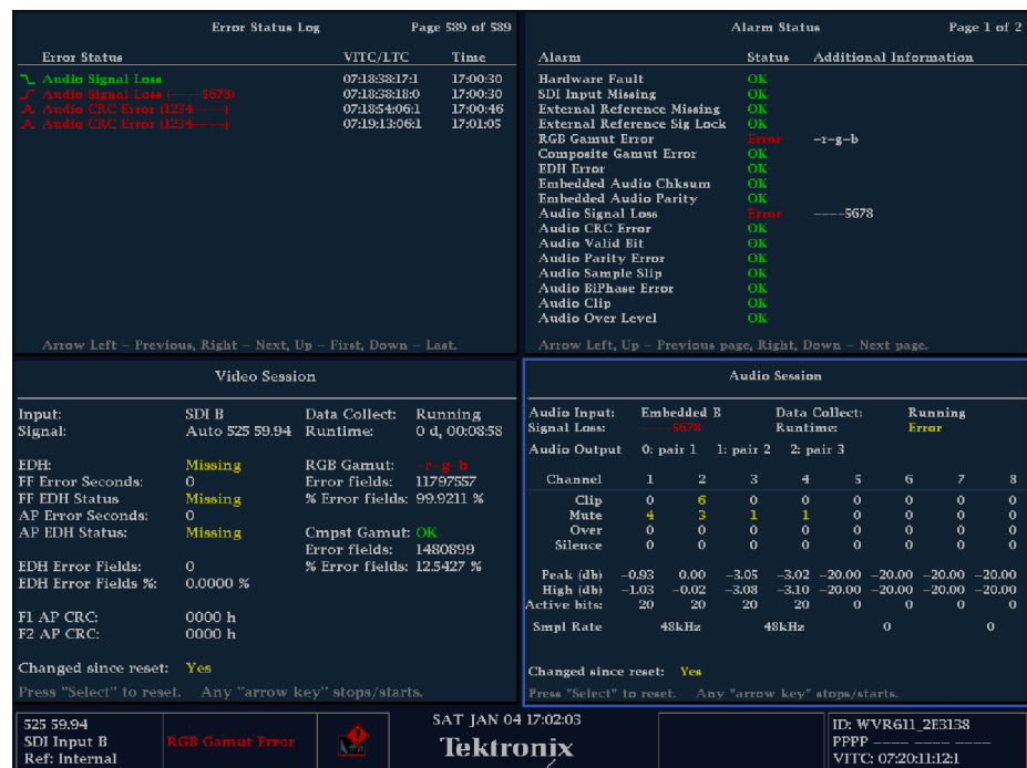
Figure 2-25: A STATUS display in all four tiles
